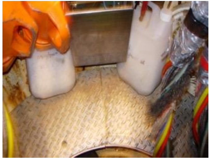
CO 2 absorbent inside a bell (Juice containers)
