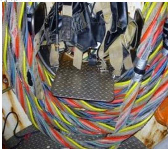
1 st and 2 nd stage releases obscured by divers umbilical
