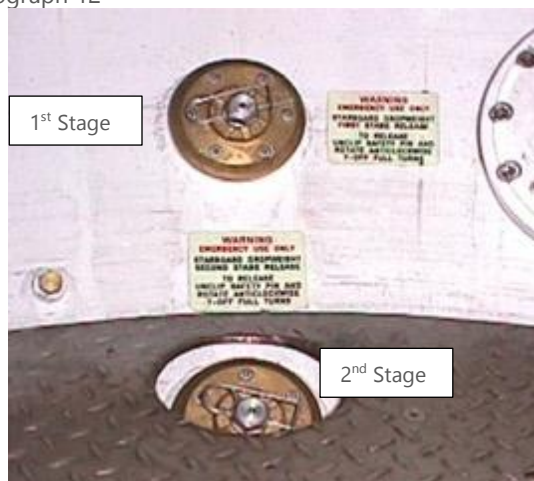
1 st & 2 nd stage release with divers umbilical removed
