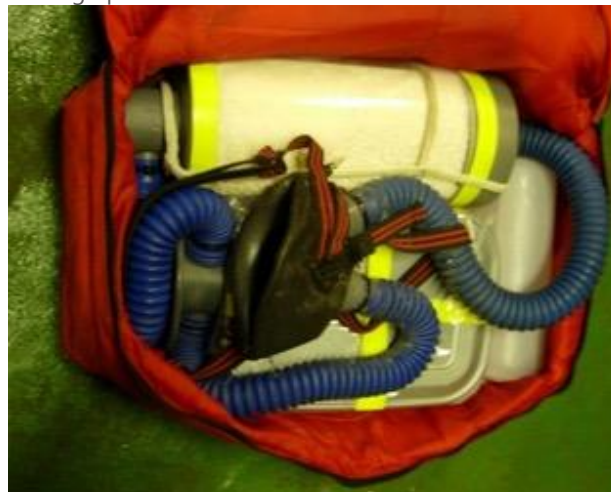
SP2 Personal scrubber and thermal regenerator
