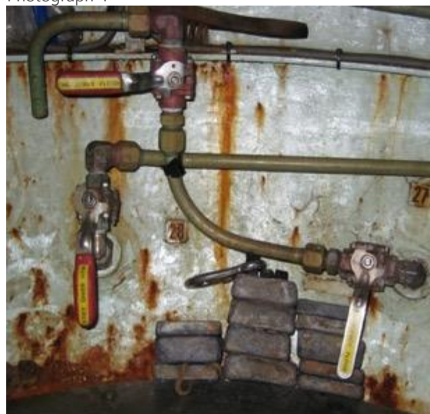
Further example of typical bell flood up arrangement. Flood up depth is below seat height and will not significantly aid the bellman with an incapacitated diver
