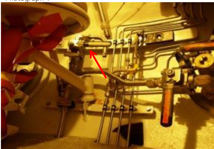
Flood up and 'goose neck' in a modern Drager designed bell. Flood up depth is below seat height and realistically will not aid the bellman with an incapacitated diver
